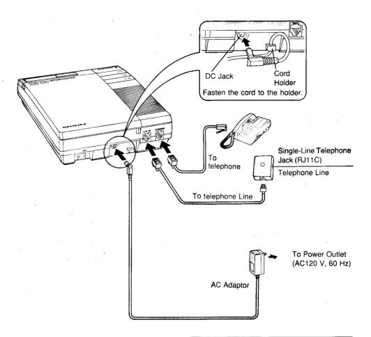
Do not connect the AC adaptor to the AC outlet before inserting the OGM and ICM tapes. (See page 6.)
